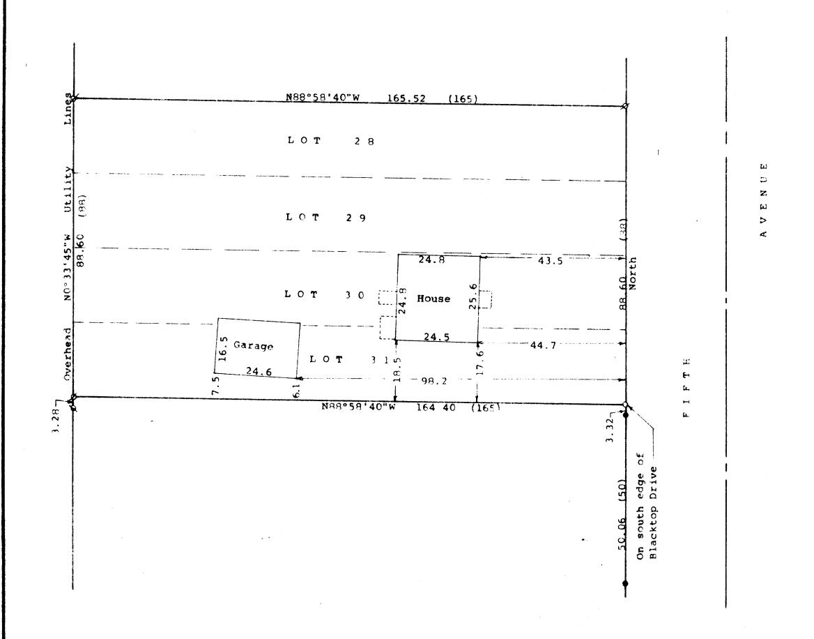
Scale - 1" = 20" $\emptyset = 3/4$ " Iron Pipe Found ⋈ = ½" Iron Pipe Found • = 1" Iron Pipe Found 0 = 3/4" Iron Pipe Set Bearings referenced to the west line of Fifth Avenue with the assumed bearing of North (0.00) = recorded distance Survey ordered by: Churchill Real Estate Walworth, WI 53184
